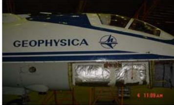
Figure 1: The SAFIRE-A spectrometer on-board the M-55 Geophysica aircraft.
